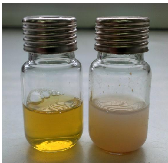
Digital photograph of a stable colloid aqueous solution of propolis /copolymer (left) and aqueous suspension of propolis (right)/.
